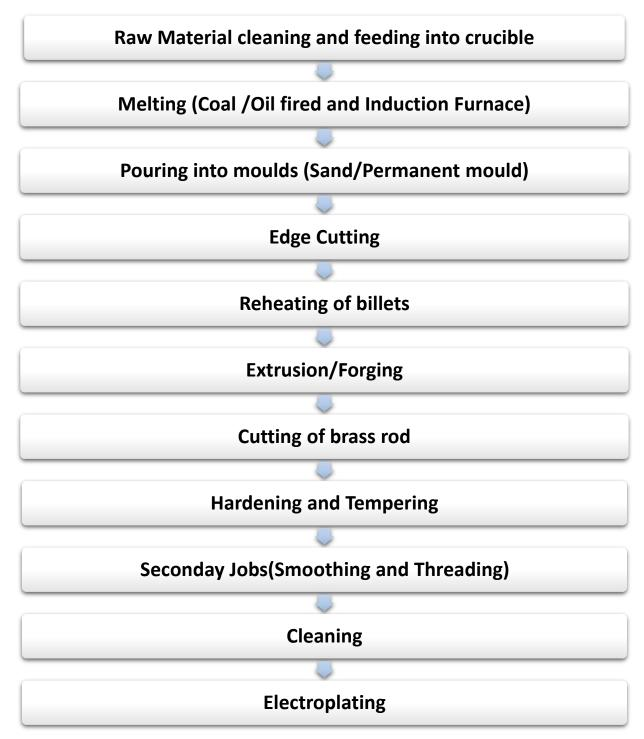
Figure 2: Typical Process Flow Chart for Brass Products in Jamnagar
