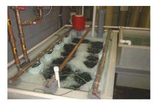
Usually, the bath is contained in metal container, lined with acid/alkali resistant membrane e.g. PVC sheet to make it insulated from electric circuit. The application of direct electric current across the bath solution causes the migration of positively charged particles (anions) towards the negative electrode (cathode) and negatively charged particles (cations) towards the positive electrodes (anode).
