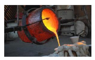
preparing the consolidated sand mould around a pattern held within a supporting metal frame and removing the pattern to leave the mould cavity with cores. The liquid brass is poured into the cavity and allowed to solidify and when it does, the product is taken out of the mould cavity, trimmed and made to shape.
