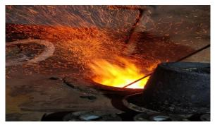
**Casting**: After melting the next step involves casting molten brass in permanent mould or sand mould, depending upon the final product of the company. Sand moulding usually involves the
